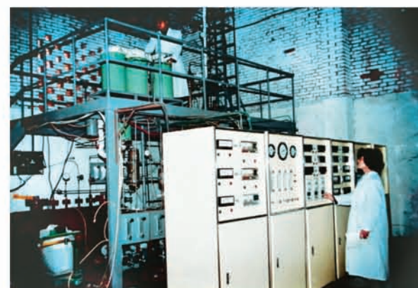
90年代甲醇制二甲醚中试装置 Pilot plant for dehydration of methanol to dimethyl ether in 1990s
