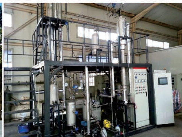
近年醋酸加氢制乙醇中试装置 Pilot plant for production of ethanol by hydrogenation of acetic ester
