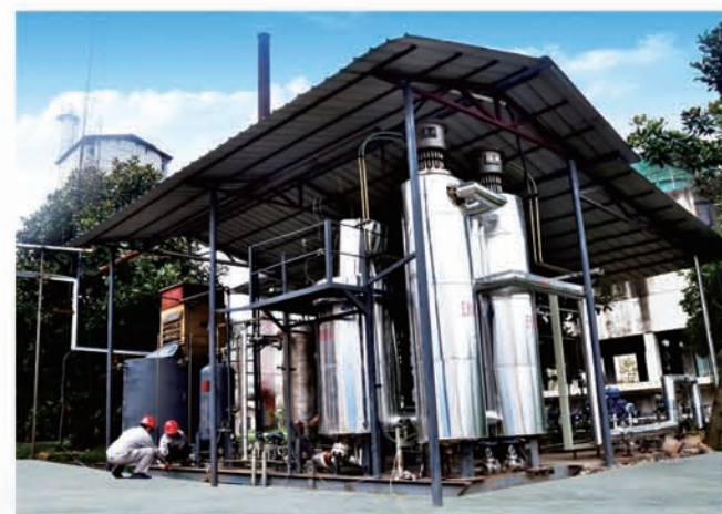
近年焦炉气甲烷化中试装置 Pilot plant for methanation of coke oven gas in recent years
