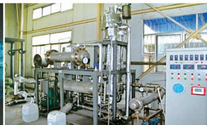
近年草酸酯加氢制乙二醇中试装置 Pilot plant for producing ethylene glycol via catalytic hydrogenation of oxalic ester in recent years
